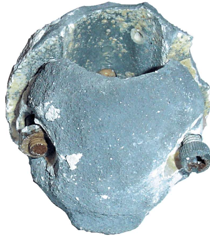
Old Zinc after 8 months (for 1" diameter shaft)
