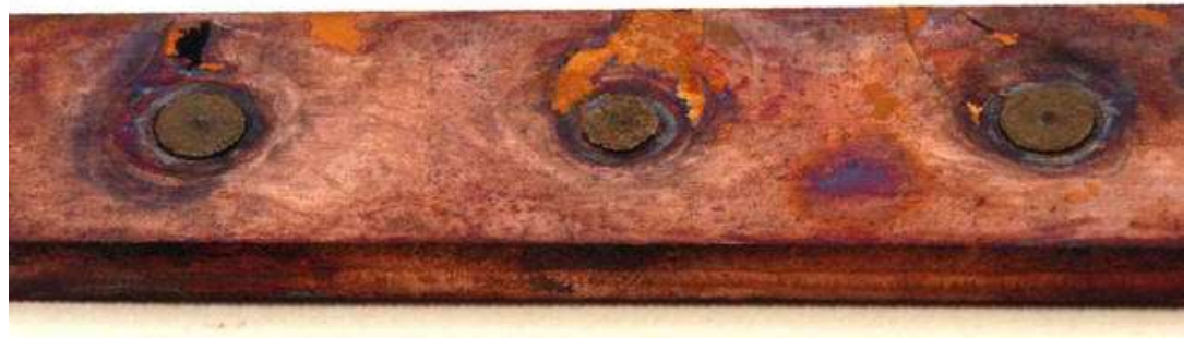
Steel rivets on a copper bar submerged in 3% sodium chloride solution after six months
