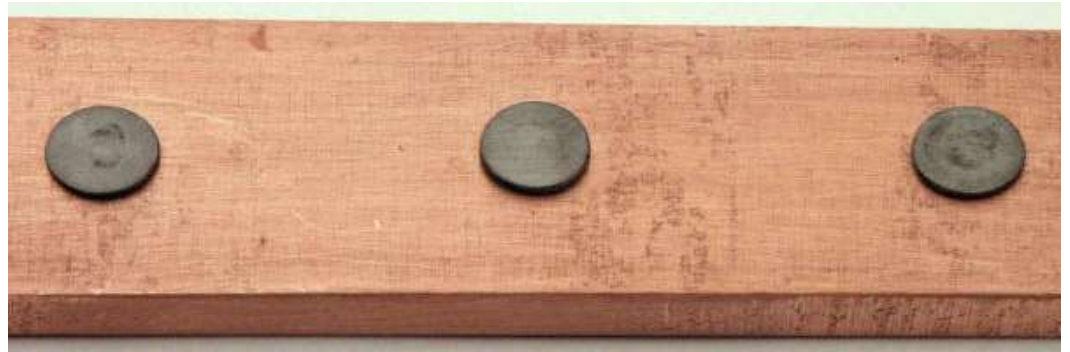
Steel rivets on a copper bar submerged in 3% sodium chloride solution at the start of the experiment
