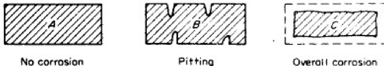
Figure 3-17 Diagrammatic representation of pitting corrosion as an intermediate stage.
