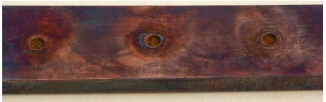
Steel rivets on a copper bar submerged in 3% sodium chloride solution after ten months
