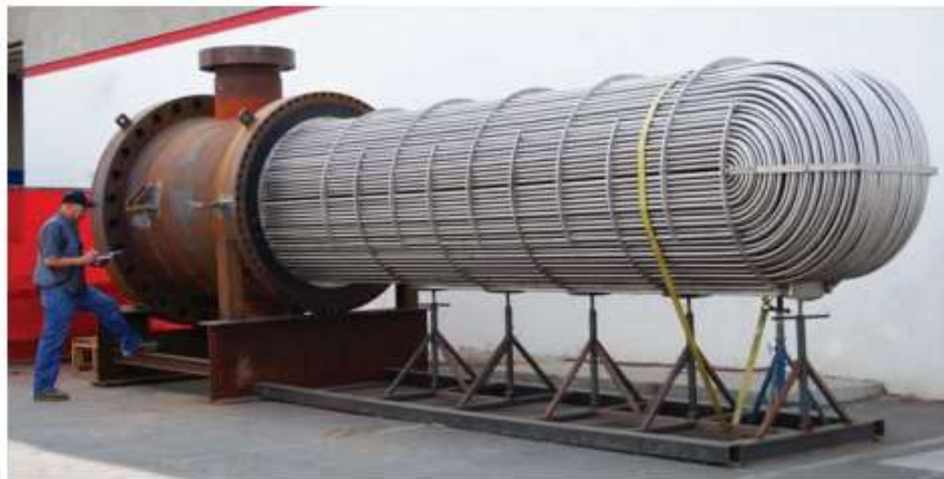
Inconel alloy 625 is suitable for seawater applications because of its excellent corrosion resistance and resistance to chloride-ion stress-corrosion cracking. Depicted here, a shell and tube heat exchanger in alloy 625. Photo: Titan.
